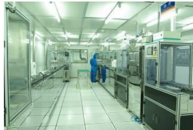
Cell-making room 100 class clean room
