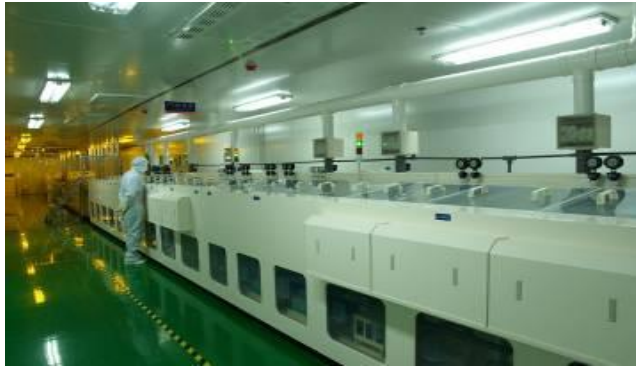
ITO glass clean line before PR coating 1000 class clean room
